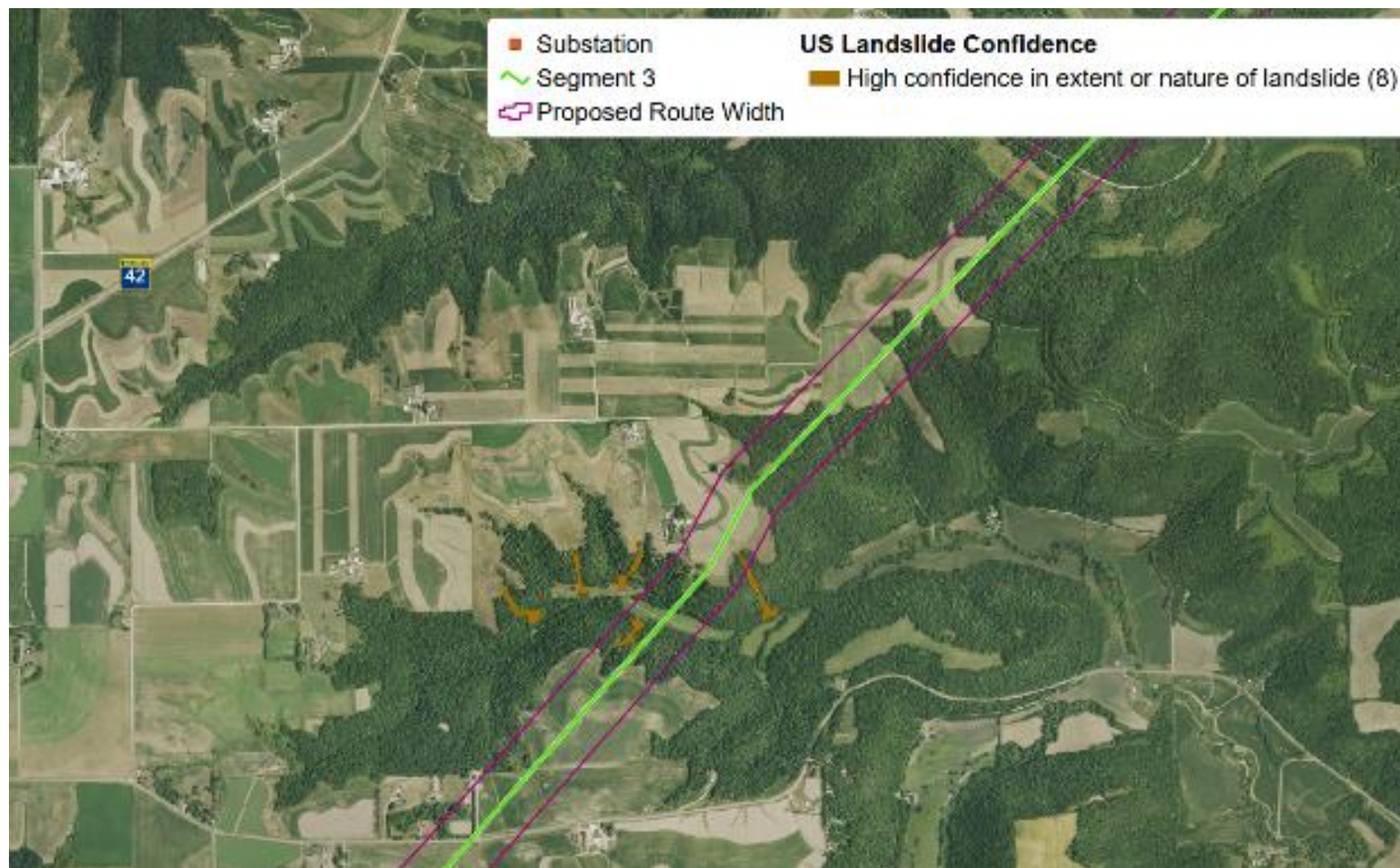
Figure 9-6 USGS United States Landslide Inventory: Activity Documented Within Segment 3 Route Width
