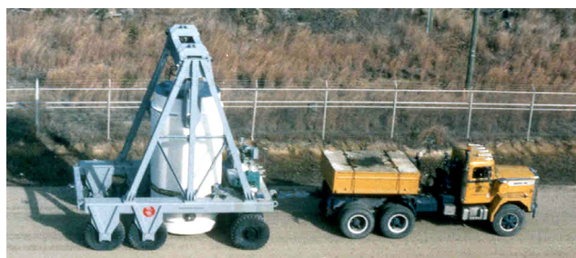
Cask transporter moves loaded spent fuel storage cask to storage pad.
