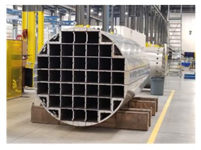
A dry fuel storage system consisting of a canister and other components provides spent fuel containment, radiation shielding, and transportation. Spent fuel assemblies are stored inside a DFS system canister. The specific vendor and spent fuel storage technology selected by Xcel Energy was the NUHOMS. 50 They are designed to store and transport spent fuel and are approved under a general license from the NRC for storage and transport. 51
