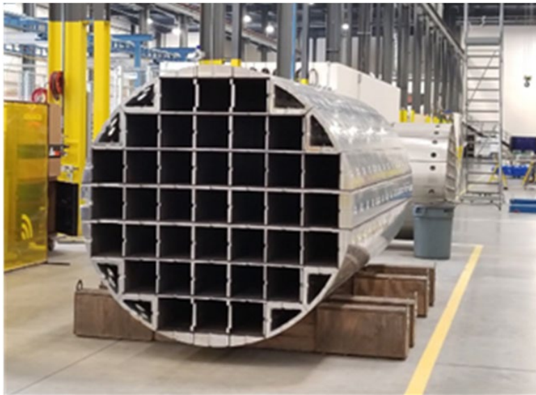
Figure 2: Spent Fuel Canister – End View with Basket for Spent Fuel Assemblies
