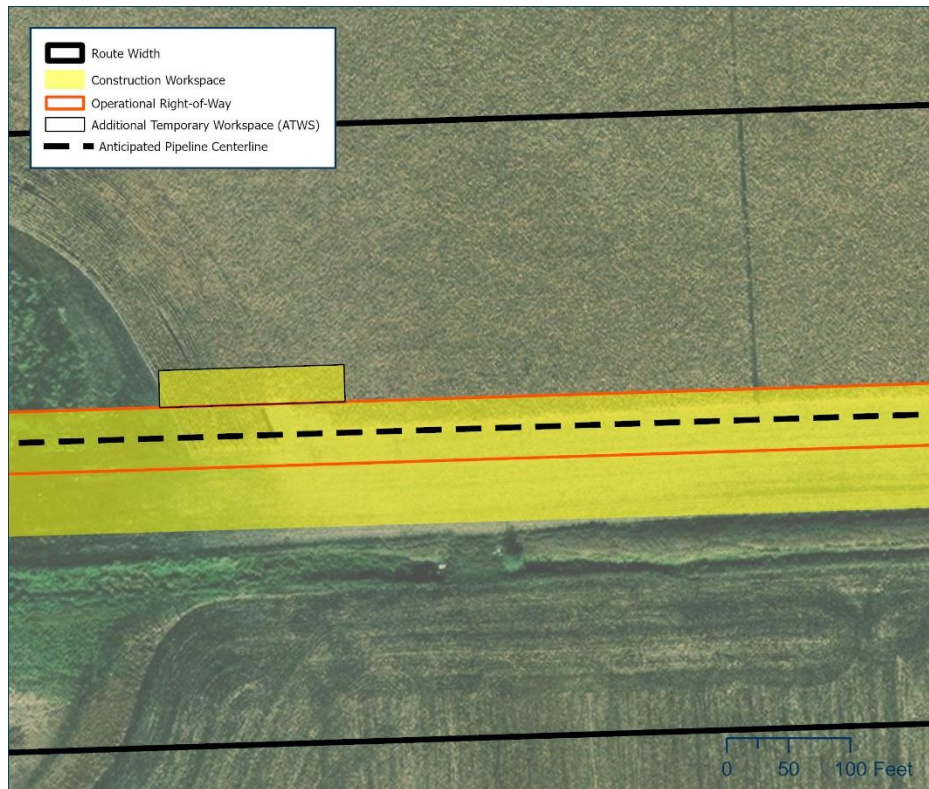
Figure 3-2 Hypothetical Route Width, Construction Workspace, and Right-of-Way Illustration
