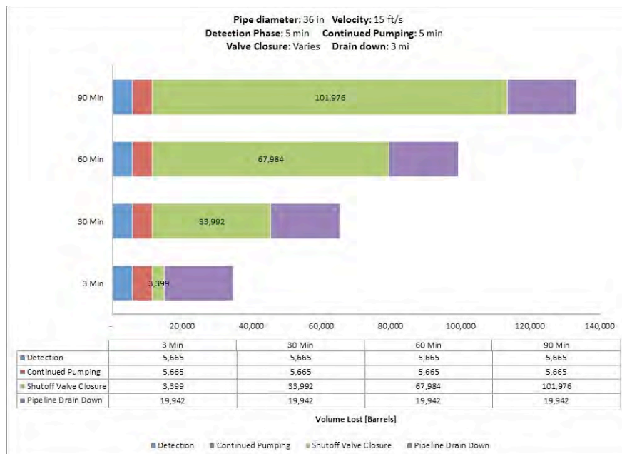
Fig. 3.82. Case Study 8A – Discharge volumes for a 36-in. hazardous liquid pipeline with a 400 psig MAOP and an elevation change of 100 ft with a 3, 30, 60, and 90 minutes block valve closure phase.
