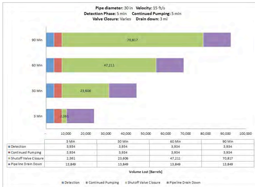
Fig. A-174. 30 Inch Pipe Diameter, 15 ft/s, 800 psi MAOP, 1000 Feet Elevation Change.
