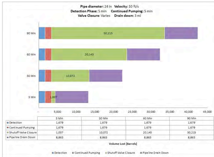
Fig. A-127. 24 Inch Pipe Diameter, 10 ft/s, 1200 psi MAOP, 100 Feet Elevation Change.
