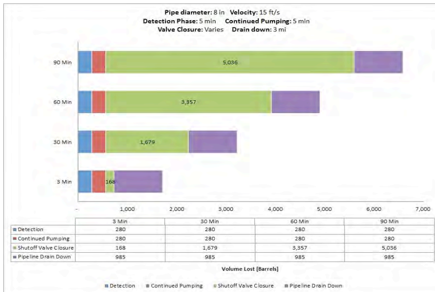
Fig. 3.79. Case Study 7B – Discharge volumes for an 8-in. hazardous liquid pipeline with a 1,480 psig MAOP and an elevation change of 100 ft with a 3, 30, 60, and 90 minutes block valve closure phase.
