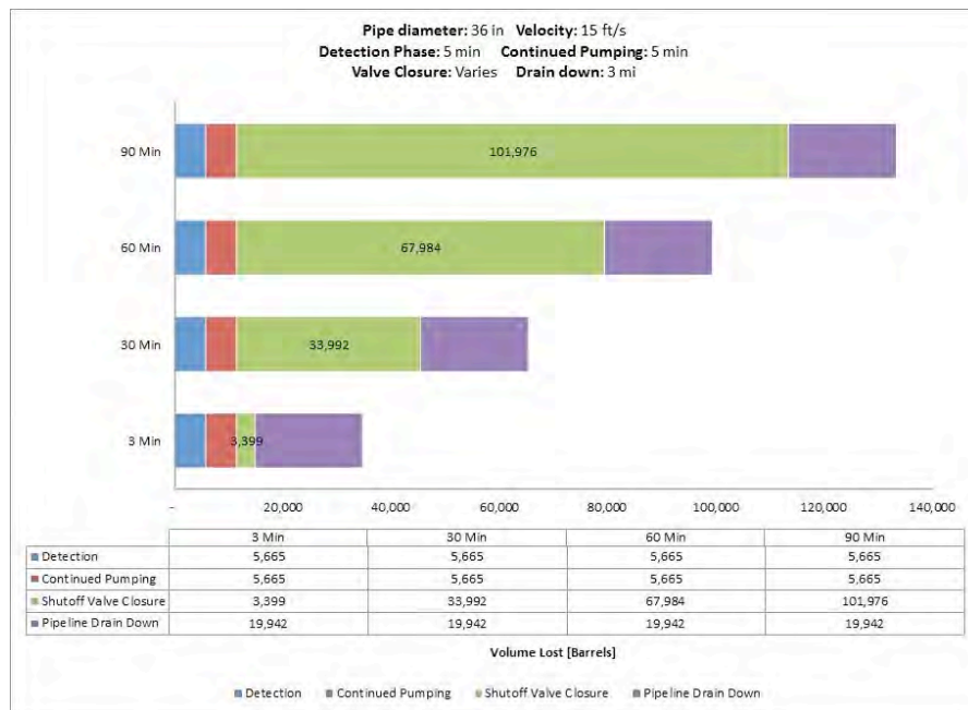
Fig. A-206. 36 Inch Pipe Diameter, 15 ft/s, 400 psi MAOP, 500 Feet Elevation Change.
