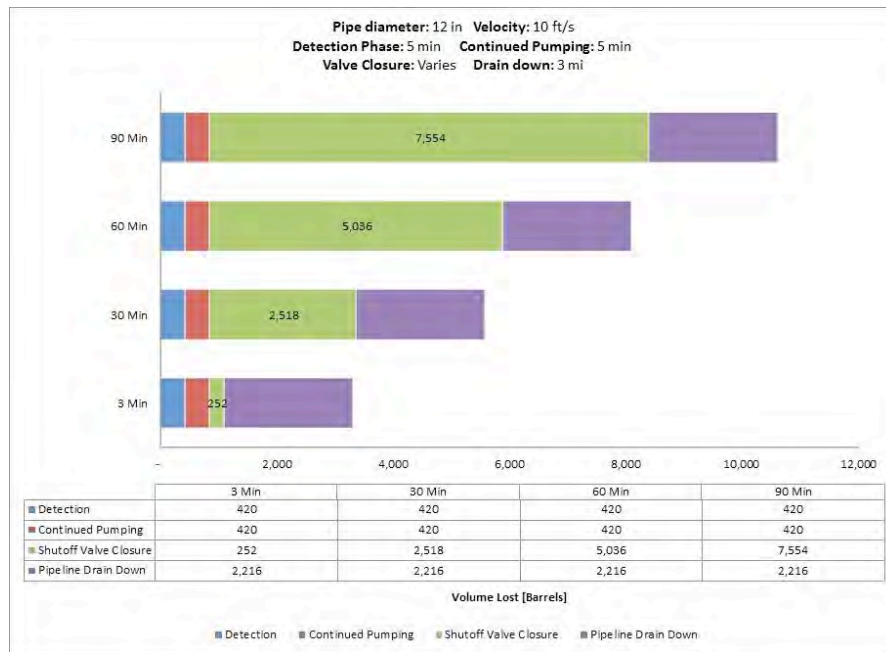
Fig. A-57. 12 Inch Pipe Diameter, 10 ft/s, 1200 psi MAOP, 1000 Feet Elevation Change.
