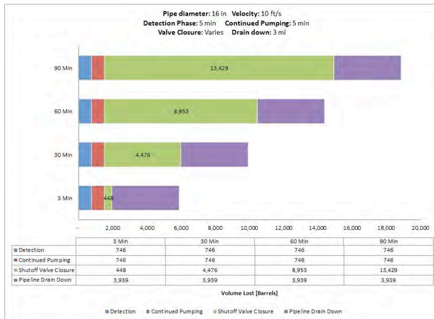
Fig. A-90. 16 Inch Pipe Diameter, 10 ft/s, 800 psi MAOP, 1000 Feet Elevation Change.
