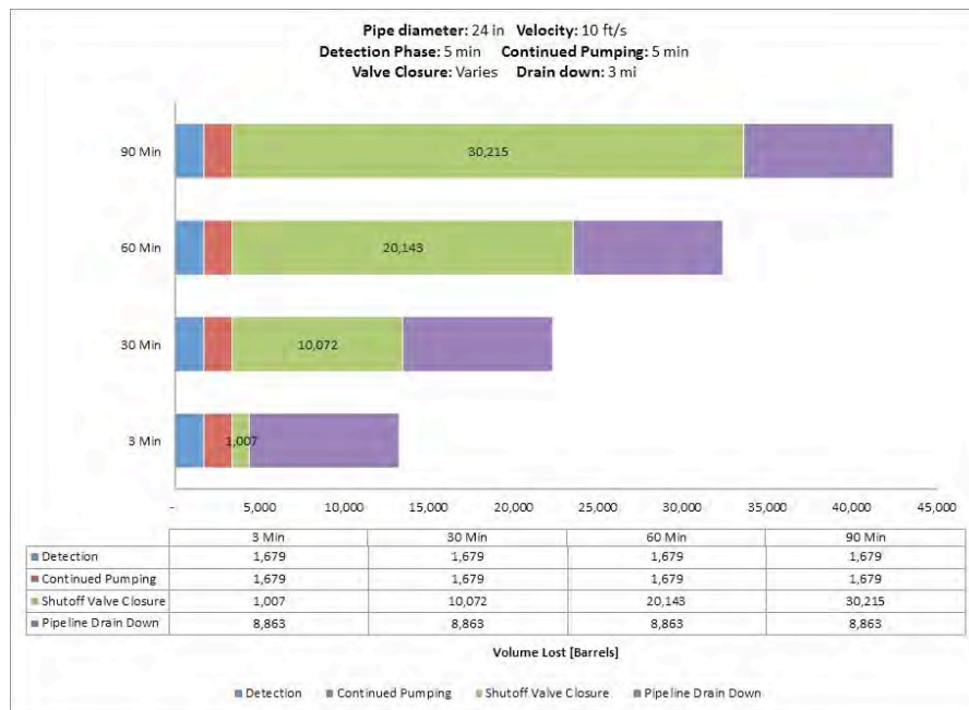
Fig. A-126. 24 Inch Pipe Diameter, 10 ft/s, 800 psi MAOP, 1000 Feet Elevation Change.
