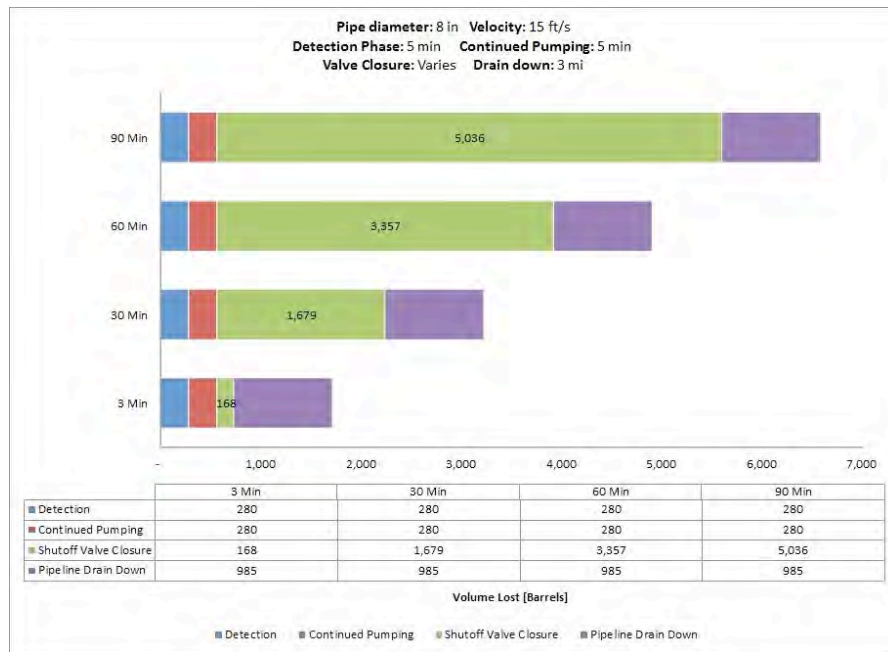
Fig. A-29. 8 Inch Pipe Diameter, 15 ft/s, 800 psi MAOP, 500 Feet Elevation Change.
