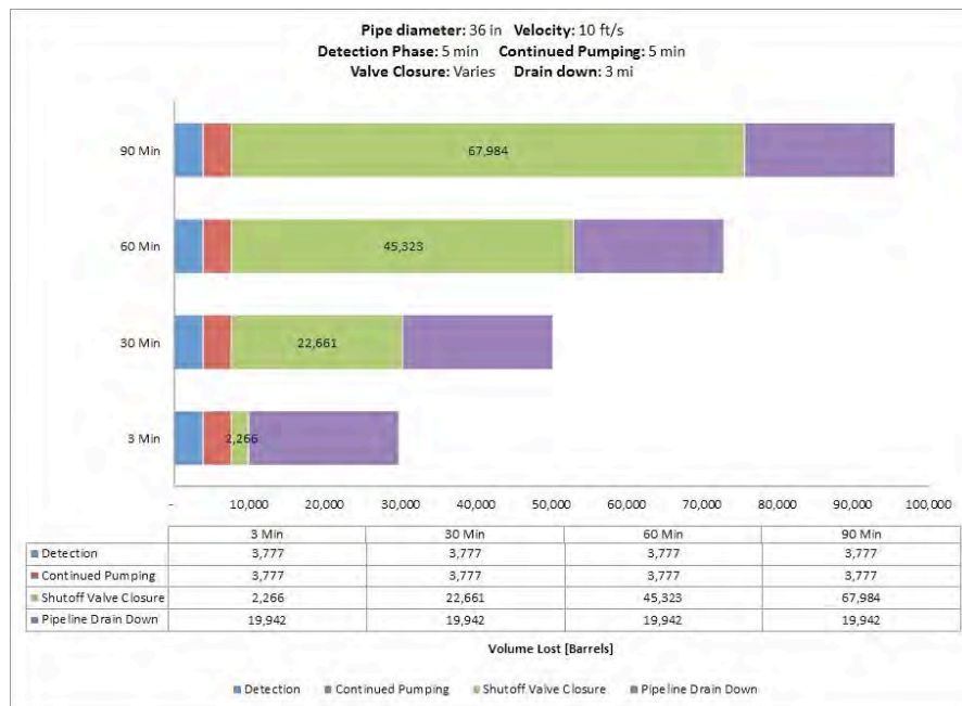
Fig. A-196. 36 Inch Pipe Diameter, 10 ft/s, 800 psi MAOP, 100 Feet Elevation Change.
