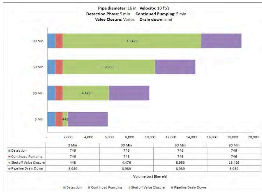
Fig. A-96. 16 Inch Pipe Diameter, 10 ft/s, 1480 psi MAOP, 1000 Feet Elevation Change.
