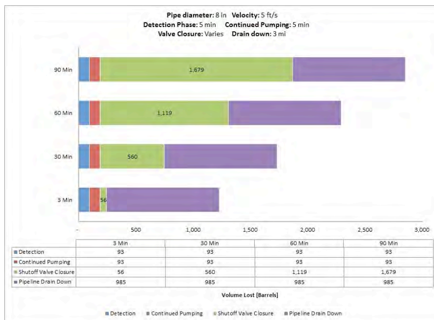
Fig. A-2.8 Inch Pipe Diameter, 5 ft/s, 400 psi MAOP, 500 Feet Elevation Change.
