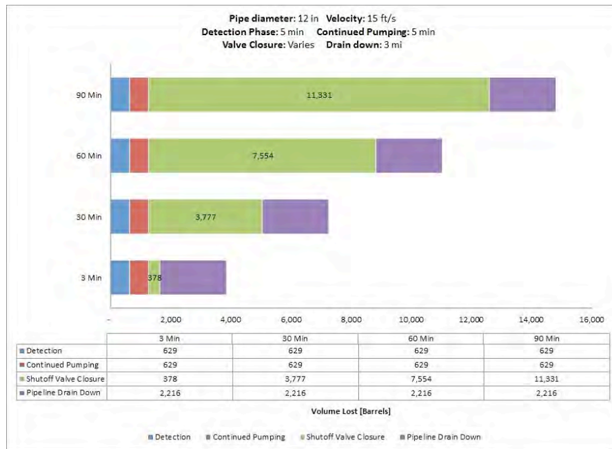
Fig. A-61. 12 Inch Pipe Diameter, 15 ft/s, 400 psi MAOP, 100 Feet Elevation Change.
