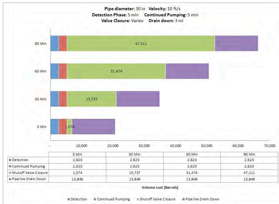
Fig. A-168. 30 Inch Pipe Diameter, 10 ft/s, 1480 psi MAOP, 1000 Feet Elevation Change.
