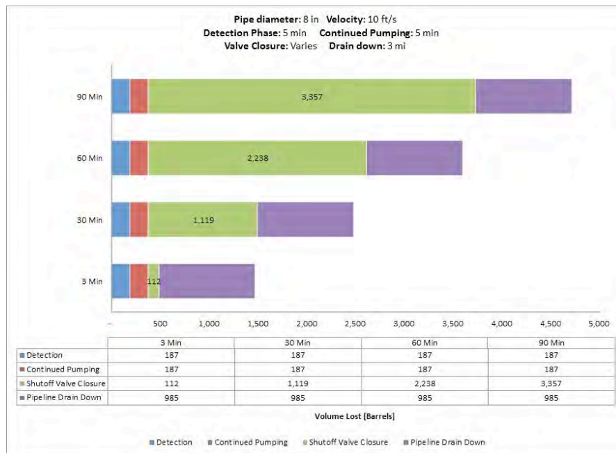
Fig. A-18. 8 Inch Pipe Diameter, 10 ft/s, 800 psi MAOP, 1000 Feet Elevation Change.
