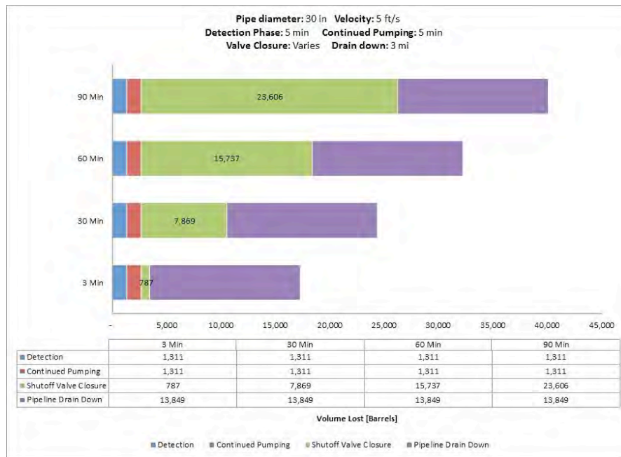
Fig. A-149. 30 Inch Pipe Diameter, 5 ft/s, 800 psi MAOP, 500 Feet Elevation Change.
