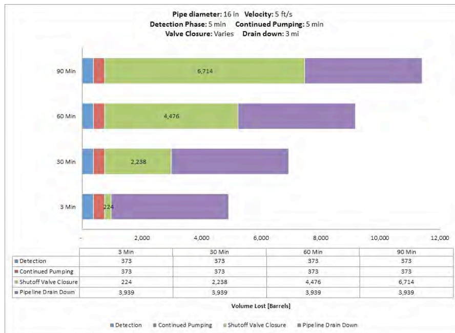
Fig. A-78. 16 Inch Pipe Diameter, 5 ft/s, 800 psi MAOP, 1000 Feet Elevation Change.
