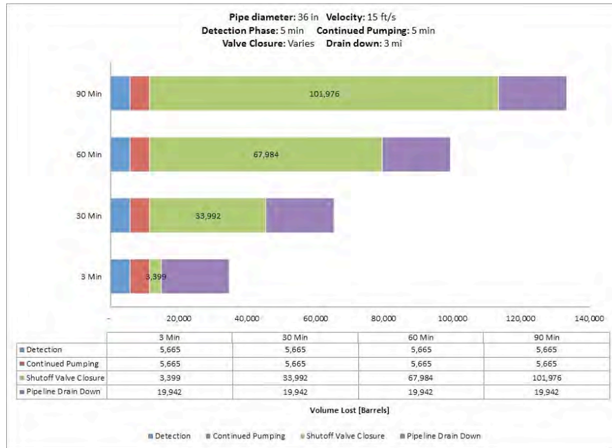
Fig. A-205. 36 Inch Pipe Diameter, 15 ft/s, 400 psi MAOP, 100 Feet Elevation Change.
