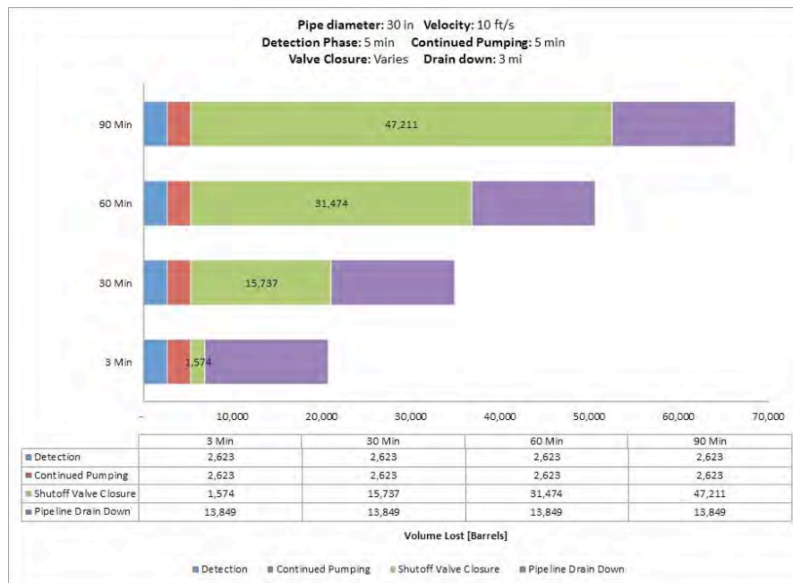
Fig. A-160. 30 Inch Pipe Diameter, 10 ft/s, 800 psi MAOP, 100 Feet Elevation Change.
