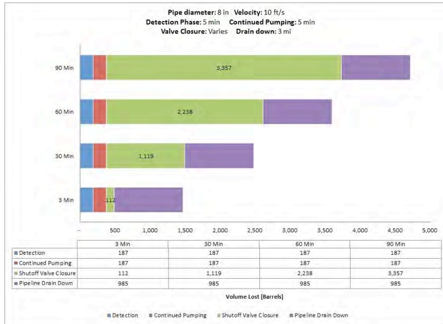
Fig. A-23. 8 Inch Pipe Diameter, 10 ft/s, 1480 psi MAOP, 500 Feet Elevation Change.
