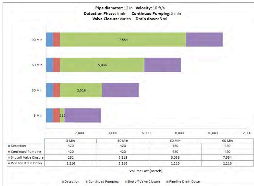
Fig. A-52. 12 Inch Pipe Diameter, 10 ft/s, 800 psi MAOP, 100 Feet Elevation Change.
