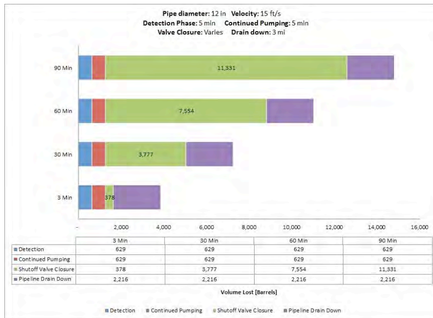
Fig. A-66. 12 Inch Pipe Diameter, 15 ft/s, 800 psi MAOP, 1000 Feet Elevation Change.
