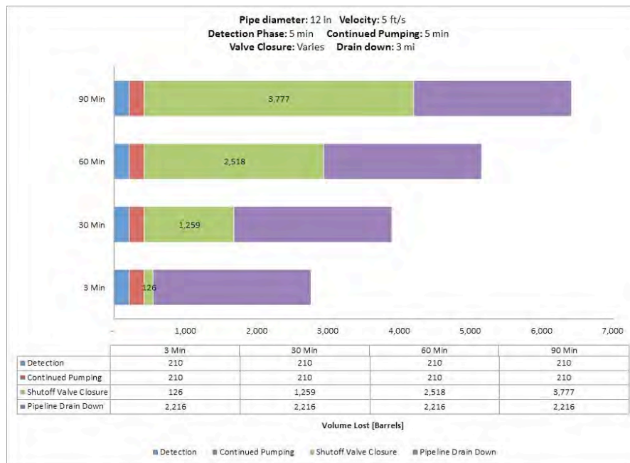
Fig. A-44. 12 Inch Pipe Diameter, 5 ft/s, 1200 psi MAOP, 500 Feet Elevation Change.
