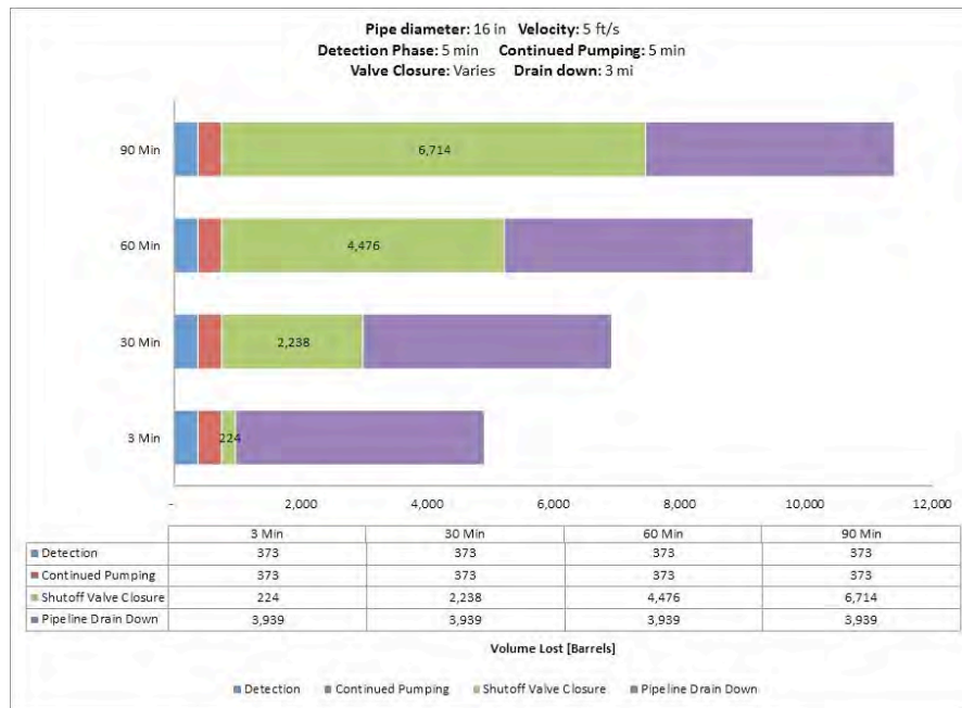
Fig. A-83. 16 Inch Pipe Diameter, 5 ft/s, 1480 psi MAOP, 500 Feet Elevation Change.
