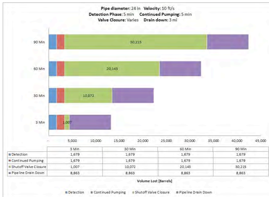
Fig. A-124. 24 Inch Pipe Diameter, 10 ft/s, 800 psi MAOP, 100 Feet Elevation Change.
