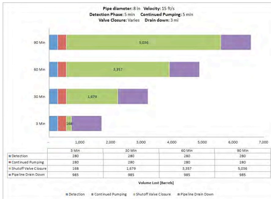
Fig. A-28. 8 Inch Pipe Diameter, 15 ft/s, 800 psi MAOP, 100 Feet Elevation Change.
