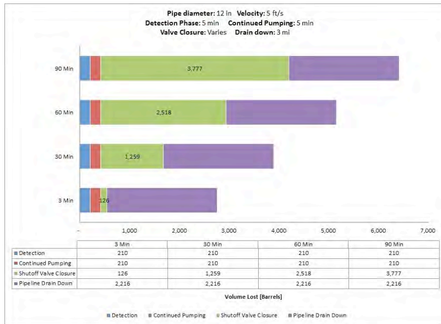
Fig. A-41. 12 Inch Pipe Diameter, 5 ft/s, 800 psi MAOP, 500 Feet Elevation Change.
