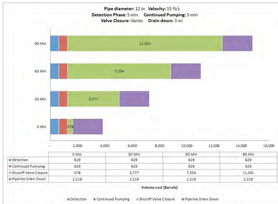
Fig. A-62. 12 Inch Pipe Diameter, 15 ft/s, 400 psi MAOP, 500 Feet Elevation Change.
