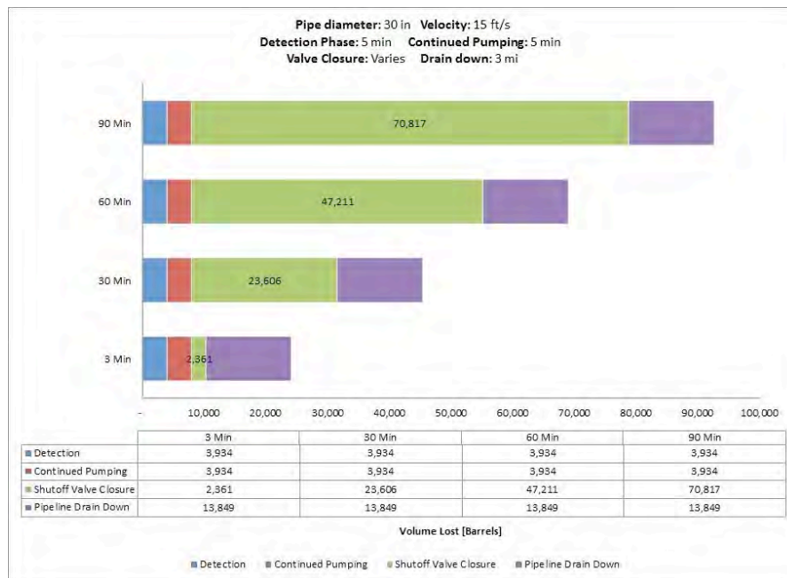
Fig. A-172. 30 Inch Pipe Diameter, 15 ft/s, 800 psi MAOP, 100 Feet Elevation Change.
