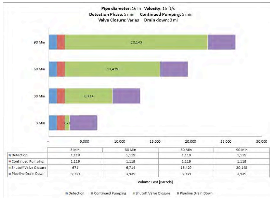
Fig. A-106. 16 Inch Pipe Diameter, 15 ft/s, 1480 psi MAOP, 100 Feet Elevation Change.
