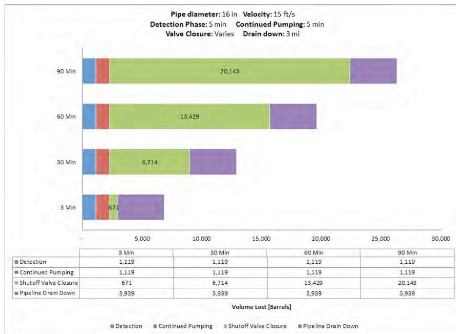
Fig. A-108. 16 Inch Pipe Diameter, 15 ft/s, 1480 psi MAOP, 1000 Feet Elevation Change.
