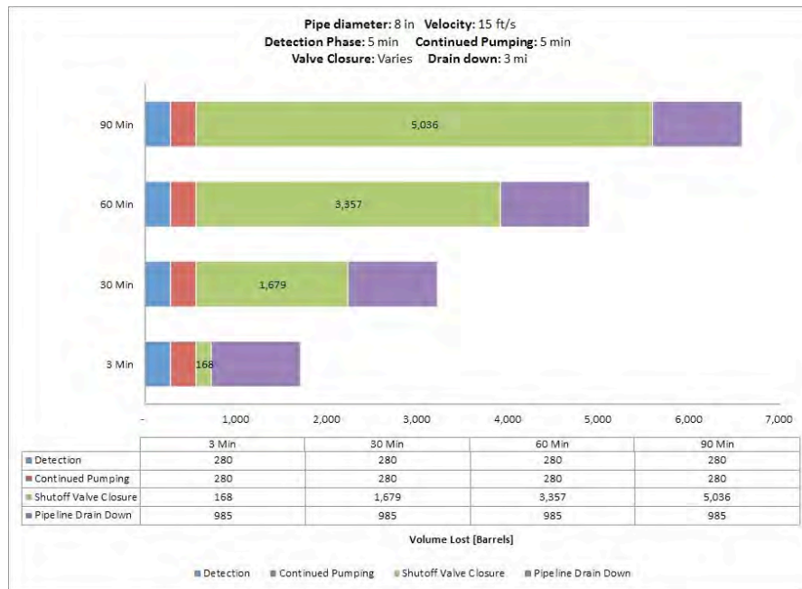
Fig. 3.80. Case Study 7C – Discharge volumes for an 8-in. hazardous liquid pipeline with a 400 psig MAOP and an elevation change of 1,000 ft with a 3, 30, 60, and 90 minutes block valve closure phase.
