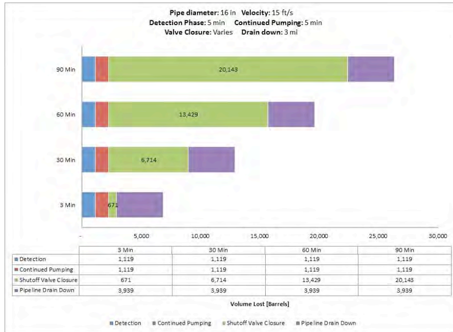
Fig. A-107. 16 Inch Pipe Diameter, 15 ft/s, 1480 psi MAOP, 500 Feet Elevation Change.
