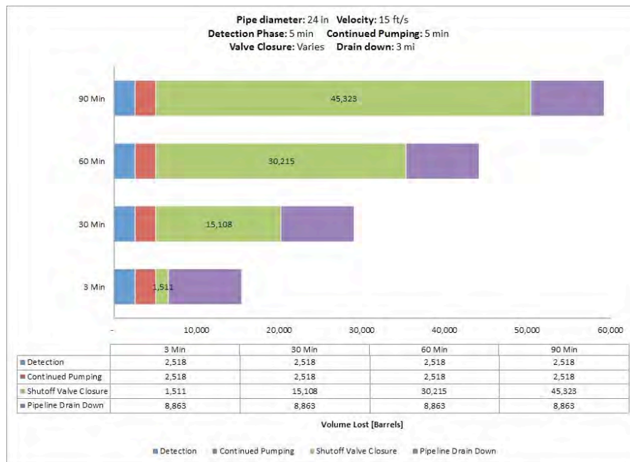
Fig. A-134. 24 Inch Pipe Diameter, 15 ft/s, 400 psi MAOP, 500 Feet Elevation Change.
