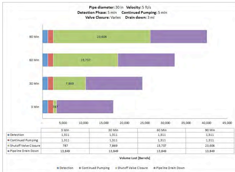
Fig. A-154. 30 Inch Pipe Diameter, 5 ft/s, 1480 psi MAOP, 100 Feet Elevation Change.
