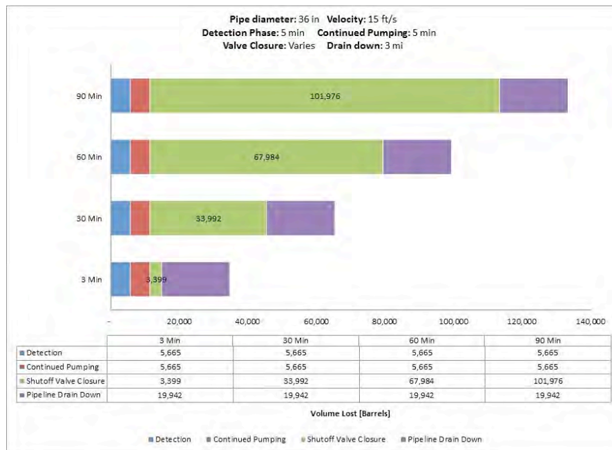
Fig. A-208. 36 Inch Pipe Diameter, 15 ft/s, 800 psi MAOP, 100 Feet Elevation Change.
