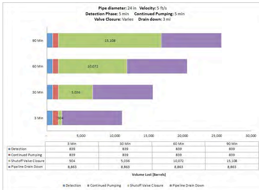
Fig. A-120. 24 Inch Pipe Diameter, 5 ft/s, 1480 psi MAOP, 1000 Feet Elevation Change.
