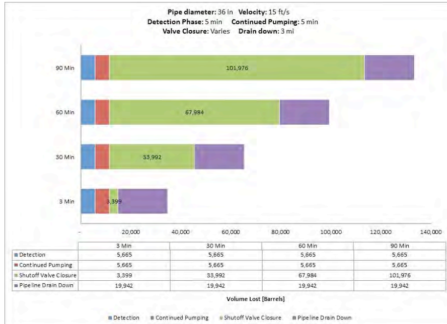
Fig. 3.83. Case Study 8B – Discharge volumes for a 36-in. hazardous liquid pipeline with a 1,480 psig MAOP and an elevation change of 100 ft with a 3, 30, 60, and 90 minutes block valve closure phase.
