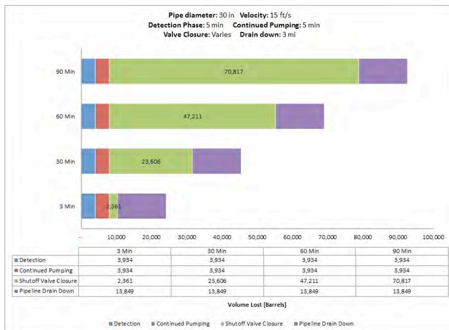
Fig. A-176. 30 Inch Pipe Diameter, 15 ft/s, 1200 psi MAOP, 500 Feet Elevation Change.
