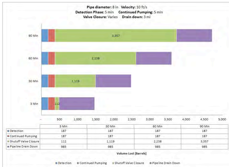
Fig. A-24. 8 Inch Pipe Diameter, 10 ft/s, 1480 psi MAOP, 1000 Feet Elevation Change.
