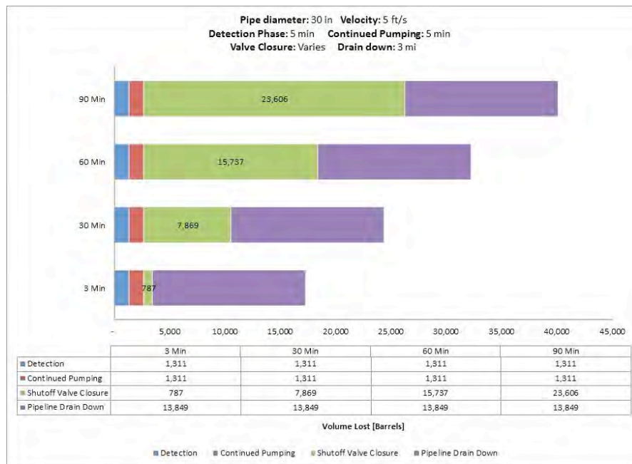
Fig. A-146. 30 Inch Pipe Diameter, 5 ft/s, 400 psi MAOP, 500 Feet Elevation Change.
