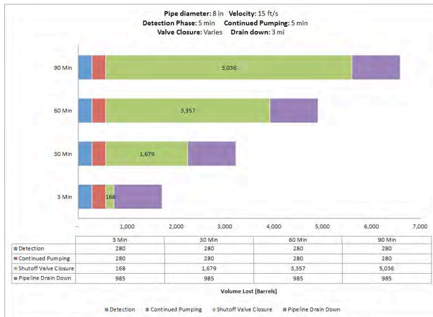
Fig. A-34. 8 Inch Pipe Diameter, 15 ft/s, 1480 psi MAOP, 100 Feet Elevation Change.
