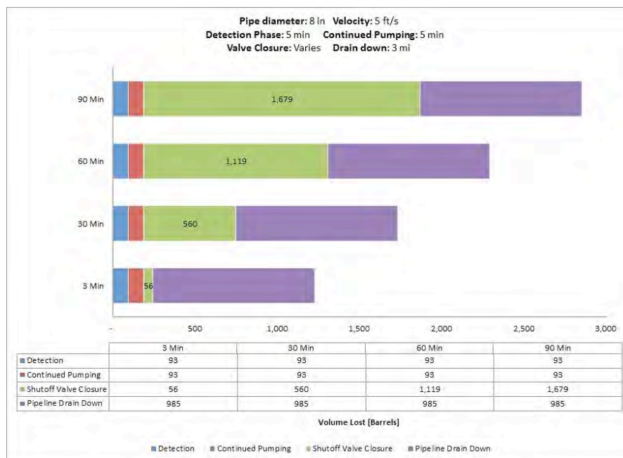
Fig. A-1.8 Inch Pipe Diameter, 5 ft/s, 400 psi MAOP, 100 Feet Elevation Change.
