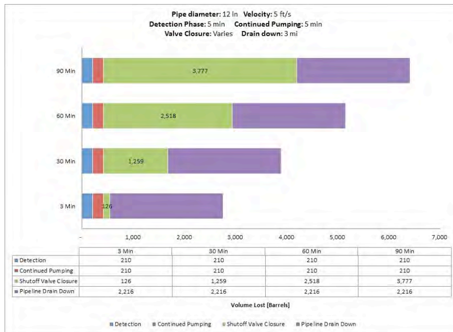
Fig. A-48. 12 Inch Pipe Diameter, 5 ft/s, 1480 psi MAOP, 1000 Feet Elevation Change.
