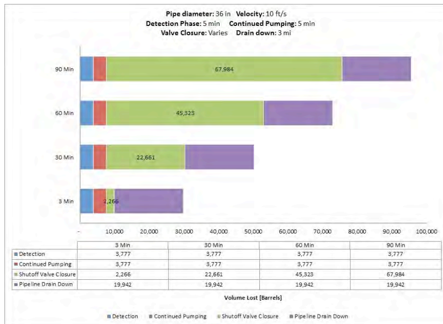
Fig. A-198. 36 Inch Pipe Diameter, 10 ft/s, 800 psi MAOP, 1000 Feet Elevation Change.
