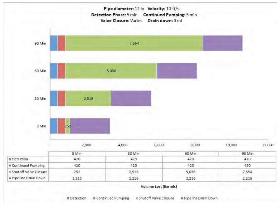
Fig. A-50. 12 Inch Pipe Diameter, 10 ft/s, 400 psi MAOP, 500 Feet Elevation Change.
