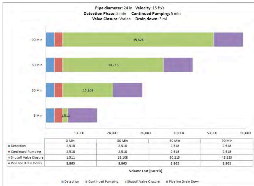
Fig. A-144. 24 Inch Pipe Diameter, 15 ft/s, 1480 psi MAOP, 1000 Feet Elevation Change.
