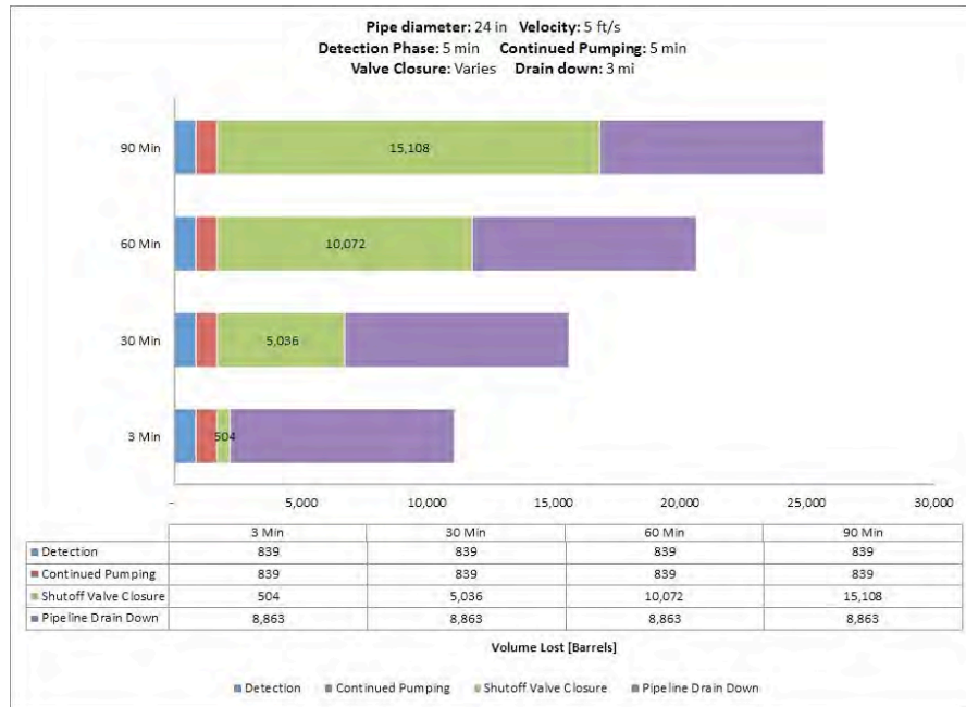
Fig. A-115. 24 Inch Pipe Diameter, 5 ft/s, 1200 psi MAOP, 100 Feet Elevation Change.
