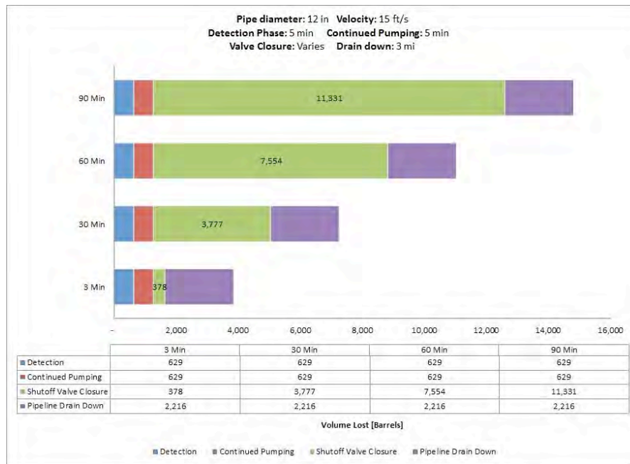
Fig. A-69. 12 Inch Pipe Diameter, 15 ft/s, 1200 psi MAOP, 1000 Feet Elevation Change.
