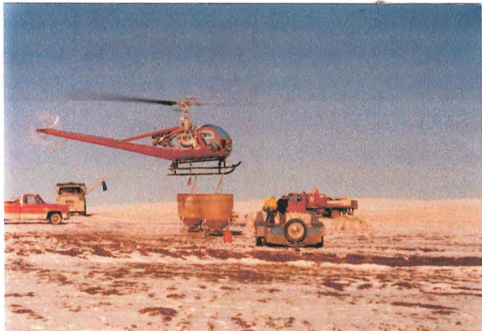
#26 Helicopter seeding crew. The helicopter carries a bucket that spreads native grass seeds on the r-o-w.
