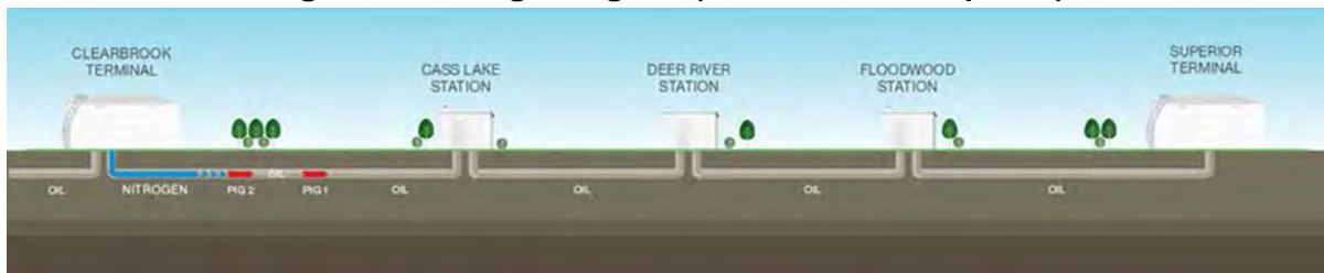
Figure 4-3: Purge Diagram (Clearbrook to Superior)
