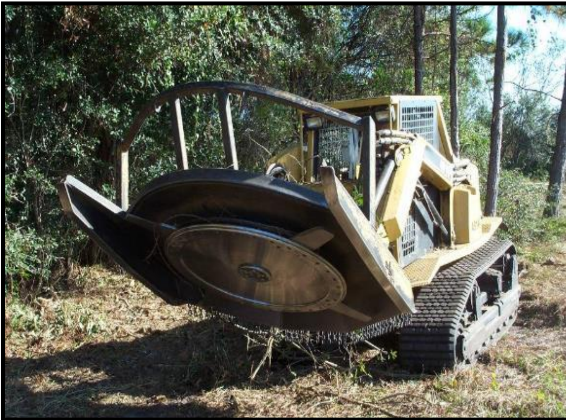
A hydro-axe will be used to efficiently mulch trees and shrubs without damaging top soil.
