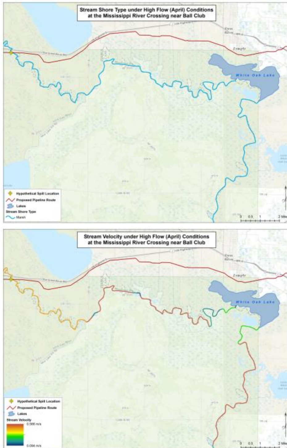
Figure 5-15 Stream Shore Type (top) and Velocity (bottom) Modeled Under High Flow Conditions for the Mississippi River Near Ball Club Release Location
