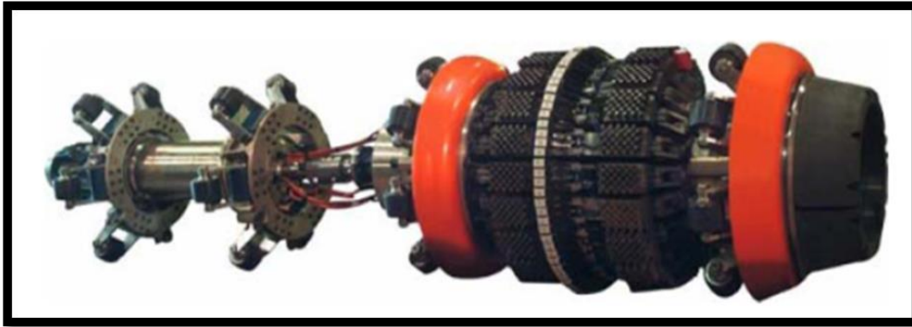
Figure 7– In-Line Inspection: Baker Hughes Vectra tool
