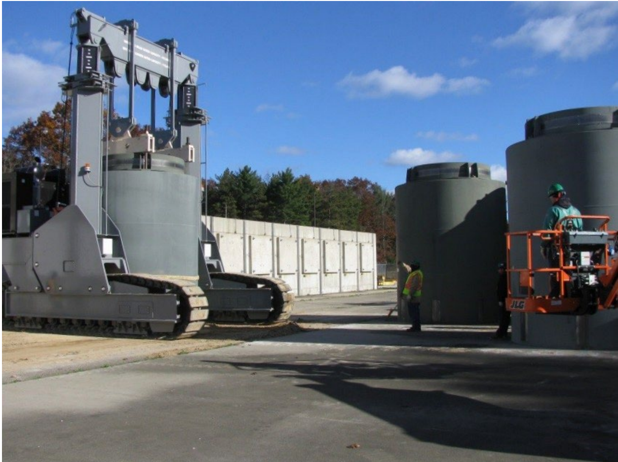
Figure C-19: Overpack and Canister Movement to ISFSI Pad Using Transporter
