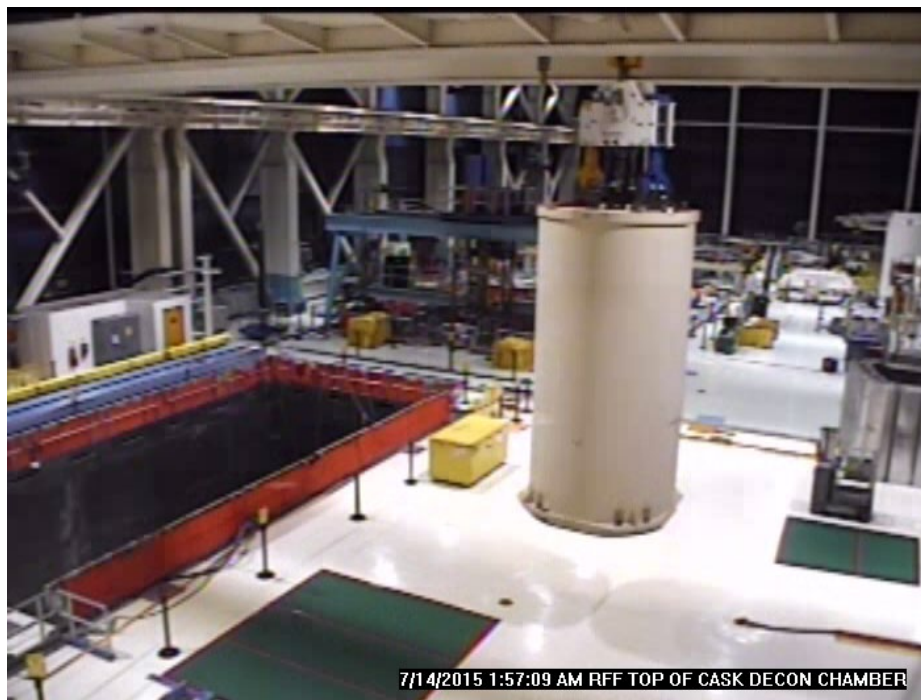
Figure C-10: Transfer Cask and Canister Movement to the Spent Fuel Pool
