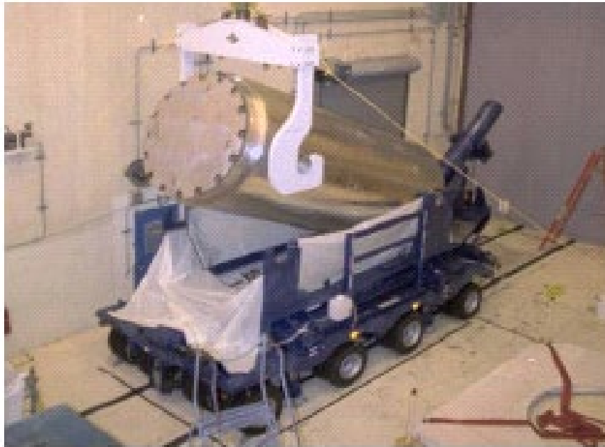
Figure C-8: Lowering Cask onto Trailer
