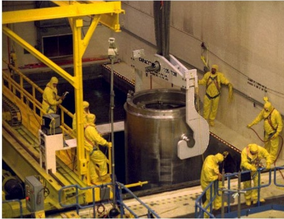
Figure C-7: Lowering Transfer Cask to Decontamination Area
