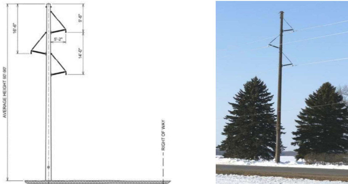
Image 4: Typical Overhead Transmission Line Structure
