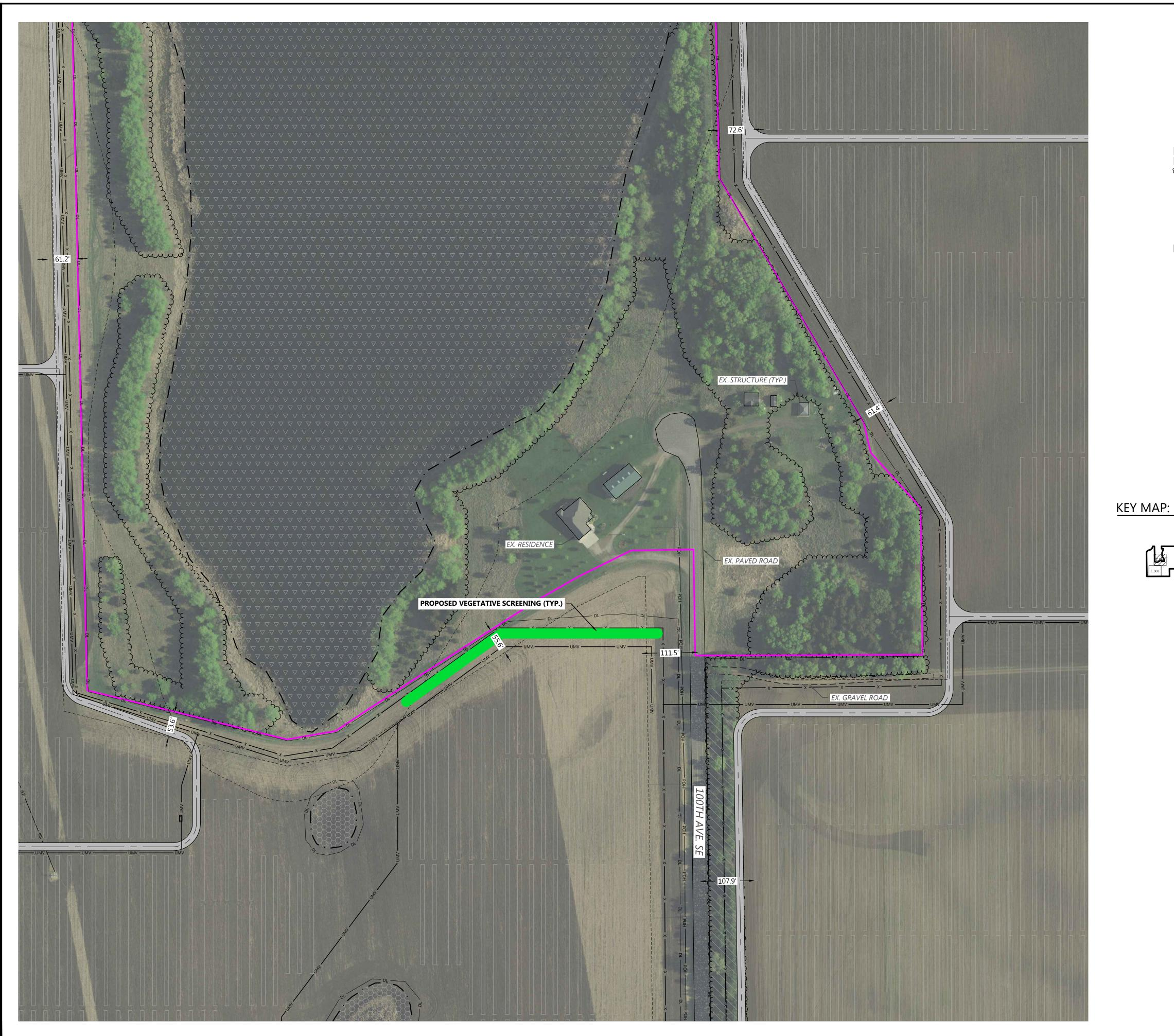
LEGEND: PROJECT BOUNDARY —— — — SECTION LINES — — RIGHT-OF-WAY LINES ————— EASEMENT LINES WWWWW EX. TREELINE EX. PAVED ROAD = = = = = EX. Gravel road EX. RAILROAD LINE ----- X ----- EX. FENCE ----- IRR ----- EX. IRRIGATION LINE POH — POH EX. OVERHEAD POWER EX. WETLAND EX. PUBLIC WATERBODY TREES TO BE CLEARED PROPOSED SOLAR ARRAY
