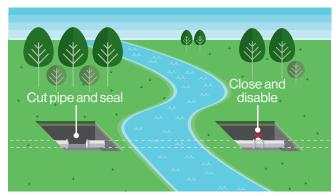
5. Segmenting the pipeline: Further isolation may be employed where necessary with the use of the permanent closure of pipeline valves or other means, including cutting and sealing.
