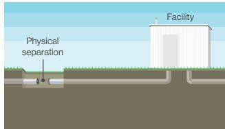
4. Disconnect the pipeline: The pipeline is physically disconnected and sealed off from the active operational facilities.
