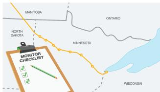
6. Monitor the pipeline right-of-way: The pipeline will continue to be monitored with regular right-of-way patrols, signs indicating location, depth of cover surveys and inclusion in "Call Before You Dig" programs.
